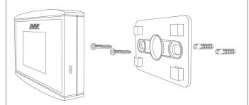
Refer to the installation manual for details, the accessories includes; wall mount bracket, screws, and wall plug. After installing the wall mount bracket, simply mount the unit onto the wall bracket and slide to lock into position.
