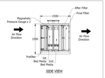
The filters arrangement for the DBS are prefilter, 2 stages of media bed followed by 2 stages of particle filters as shown below:
